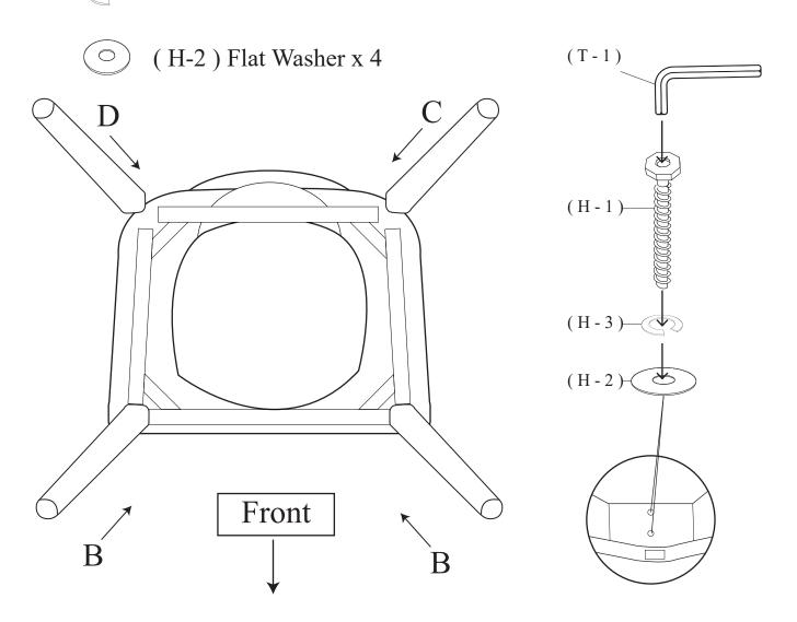
Insert Rear Legs (C),(D) into position. Secure the legs using KD Bolts (H-1), Spring Washers (H-3) and Flat Washers (H-2), stacking the hardware in the order as show. Fully engage all bolts but do not tighten them until Step 3.
